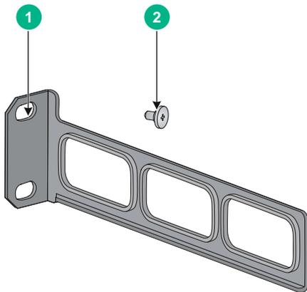
(1): 安装后挂耳到机柜立柱方孔条的螺钉孔
